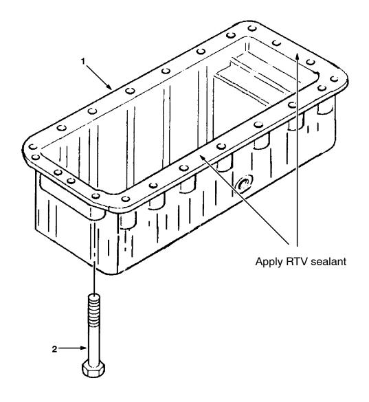
FIG. 1 - New Oil Pan Assembly
